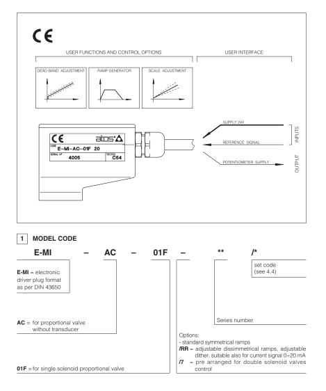
E-MI-AC drivers control the current to the solenoid of Atos proportional valves without pressure or position transducer, regulating the spool position, the flow or the pressure according to the electronic reference signal.
